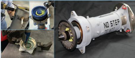
The H-60 Drive Shaft Assemblies are dynamically balanced shaft sections that transmit torque from the main transmission to the Intermediate and Tail Gear Boxes. Unique to the SH-60 variant is the Pylon Disconnect Drive Shaft Assembly that enables the folding of the Tail Plyon.
