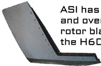
ASI has capability for repair and overhaul of main and tail rotor blades and tip caps for the H60/S70 platforms.
